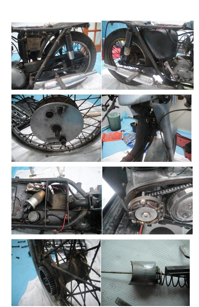
When the repainted black bits arrived back, assembly began with new rear shocks and steering races.
